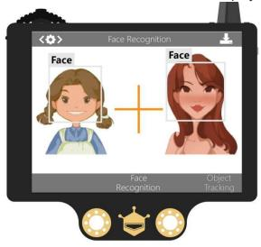
Align the "+" in the center of the HUSKYLENS screen with the face that needs to be learned, short press the "learning button" to complete the learning. If the same face is recognized, a blue frame will appear on the screen and display "Face: ID1". This shows that HuskyLens has learned the face and can recognize it now.
