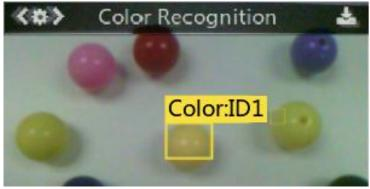
**Note:** Color recognition is greatly affected by ambient light. Sometimes HuskyLens may misidentify similar colors. Please try to keep the ambient light unchanged. In the process of using color paper card, you can put a piece of white paper under the paper card to reduce the influence of ambient light on color recognition.
