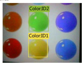
When multiple blocks of the same color appear, the separated color blocks cannot be recognized at the same time, and only one block can be recognized at one time.
