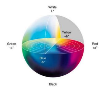
In our usual use of color recognition, the hue and saturation in the color attributes of the same module are fixed, but the brightness will change due to the influence of the ambient brightness, so you must try to ensure that when using the HUSKYLENS color recognition function, the environment brightness during learning and recognition is consistent with that during actual work.
