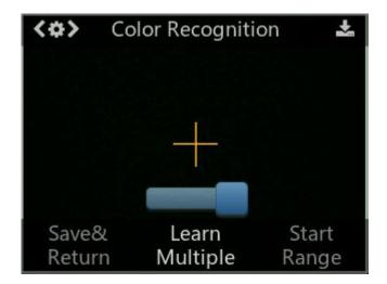
4. Dial the function button to the left until "Save & Return" shows. And the screen prompts "Do you want to save the parameters?" Select "Yes" in default, now short-press the function button to save the parameters and return automatically.
