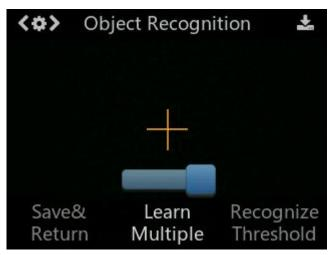
Dial the "function button" to the left and select "save & return", short press "function button". It will display "Do you want to save the parameters?", and "yes" is the default one. Short press the "function button", the data will be saved, and it will automatically return to the object recognition mode.
