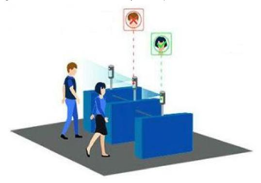
This project uses the function of HUSKYLENS to recognize multiple faces, and implements face recognition access control by performing different operations based on different recognition results. When a stranger is recognized, an alarm will sound; when a family member is recognized, the door will open automatically.
