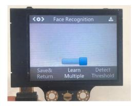
4. Dial the function button to the left until "Save & Return" shows. And the screen prompts "Do you want to save the parameters?" Select "Yes" in default, now short-press the function button to save the parameters and return automatically.
