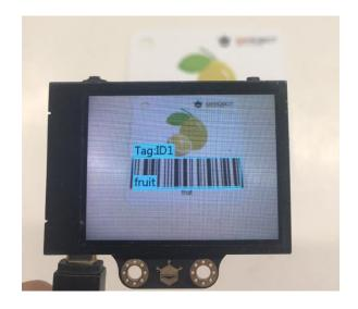
In this project, we are going to learn multiple barcodes. Therefore, we need to short press the "Learning Button" before the countdown ends. Then, point the "+" at the second barcode, pressing or holding the "Learning Button" to complete this learning, and so on.
