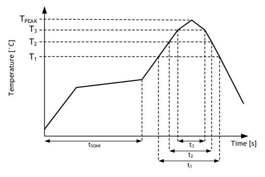
The detailed settings for the reflow profile are shown in the table below.
