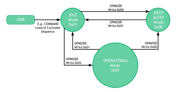
**Note:** When the active gas sensing OPMODE (e.g. 0x02 = STANDARD) is running, new data is notified either via the interrupt (INTn) or by polling the DATA\_STATUS register. The output of the gas sensing OPMODEs are presented in the DATA\_XXX registers which can be read at any time.
