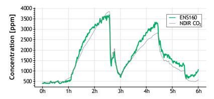
The ENS160 reverses the proportional correlation of VOCs and  $CO_2$ , by providing a standardized output signal in ppmCO<sub>2</sub>-equivalents from measured VOCs plus hydrogen, thereby adhering to today's  $CO_2$ -standards, as shown opposite: ENS160-based equivalent  $CO_2$  estimate vs.  $CO_2$ , detected by an NDIR-sensor during two consecutive meeting sessions, interrupted by a lunch-break.
