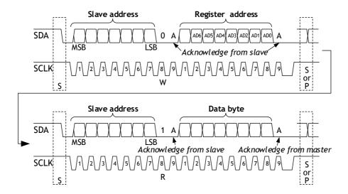
Figure 13: I<sup>2</sup>C Auto-Increment Read Operation
