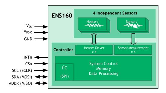
The *Heater Driver* controls the sensor operating modes and provides power to the *heaters* of each individual sensor element. During operation the heater driver regulates the heaters to their individual set-points.
