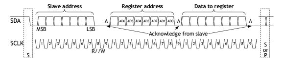
Figure 15: I<sup>2</sup>C Auto-Increment Write Operation
