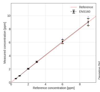
The ENS160 exhibits an excellent measurement accuracy and device-to-device variation.
