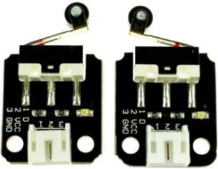
Two black proximity sensors are shown side-by-side. Each sensor has two metal detection heads extending from the top and a small PCB with two pins labeled P16 and P13.                                           | 碰撞传感器类似于按钮，可以检测到是否碰撞到障碍物。左侧碰撞传感器引脚为 P16、右侧碰撞传感器引脚为 P13。                           |
