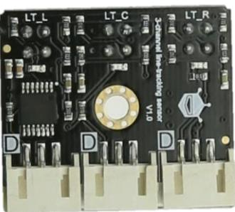
A photograph of the line tracking sensor module. It is a rectangular PCB with three infrared sensor heads labeled LT_L, LT_C, and LT_R. The PCB also has a central microcontroller and some other components.    | 巡线传感器帮助机器人进行白线或者黑线的跟踪，可以检测白背景中的黑线，也可以检测黑背景的白线。共三个检测头，但只用到了左右两个，左侧引脚为 P15、右侧为 P14。 |
