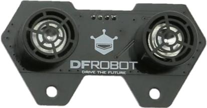
A photograph of the ultrasonic sensor module. It is a black hexagonal base with two circular transducers mounted on it. The DFRobot logo is printed on the base.                                                 | 发射端发射出超声波，超声波遇到障碍物反射回接收端。超声波传感器发射端引脚为 P1、接收端引脚为 P2。                               |
