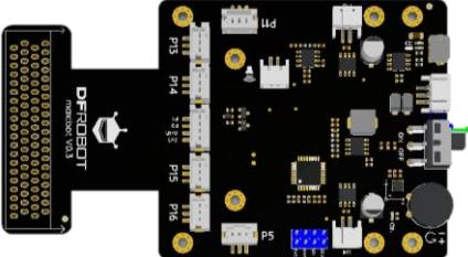
A photograph of the Max:bot expansion board. It is a black printed circuit board with various electronic components, connectors, and a central microcontroller chip. The DFRobot logo is visible on the left side. | 电路板可以搭载 Max:bot 的超声波传感器、喇叭等多种传感器和驱动器。                                             |
