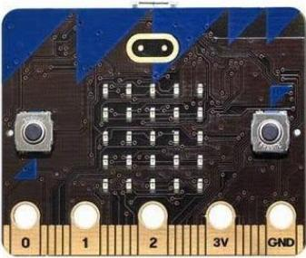
A photograph of the Micro:bit single-board computer. It features a central circular BBC logo, two small buttons on the sides, and a row of five pins at the bottom labeled 0, 1, 2, 3V, and GND.                   | Micro:bit 是一款由英国 BBC 设计的 ARM 架构的单片机，板载蓝牙，加速度计，电子罗盘，三个按钮， 5×5 LED 点阵。              |
