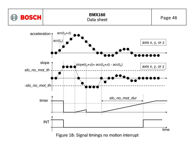
The figures below show the differences in the logic operation between the slow-motion and nomotion interrupt functionality.
