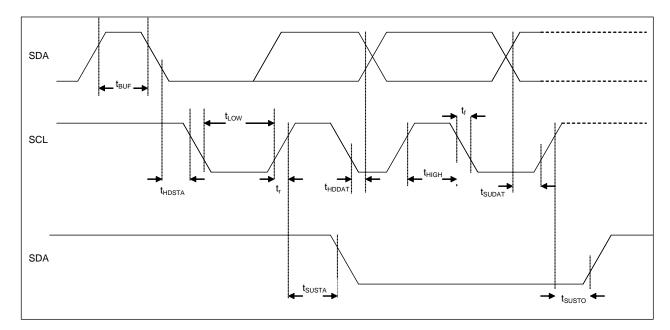
Figure 27: I<sup>2</sup>C timing diagram
