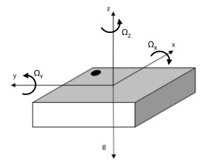
Figure 36: Definition of sensing axes orientation
