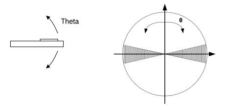
Figure 14: Flat orientation angles
