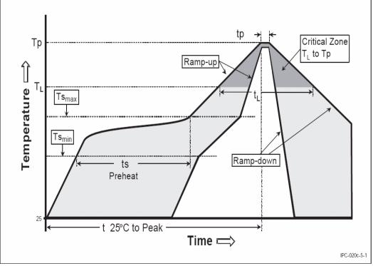
Figure 39: Soldering profile
