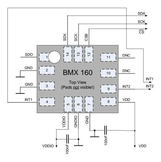
Figure 33: Only SPI 3-wire
