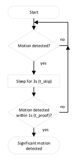
Figure 7: Block diagram of significant motion interrupt algorithm
