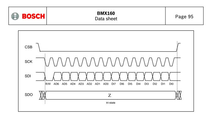
Figure 23: 4-wire basic SPI write sequence (mode "11")
