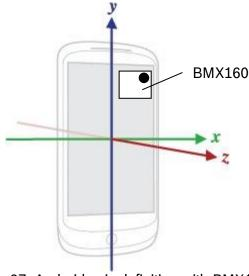
Figure 37: Android axis definition with BMX160
