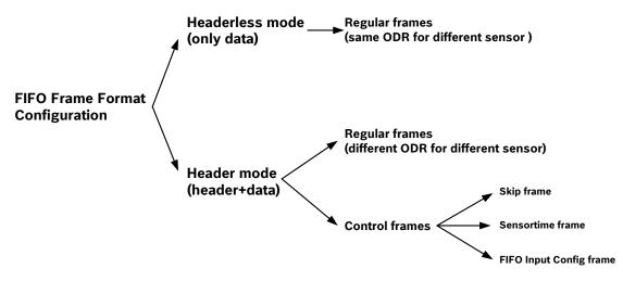
Figure 5: FIFO frame configurations
