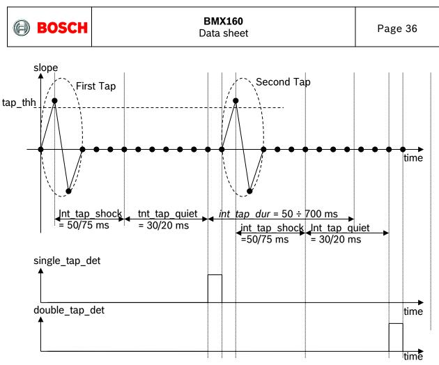
Figure 8: Tap detection interrupt
