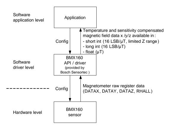
Figure 3: Calculation flow of magnetic field data from raw BMX160 register data
