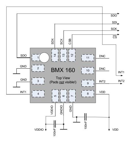
Figure 34: Only SPI 4-wire
