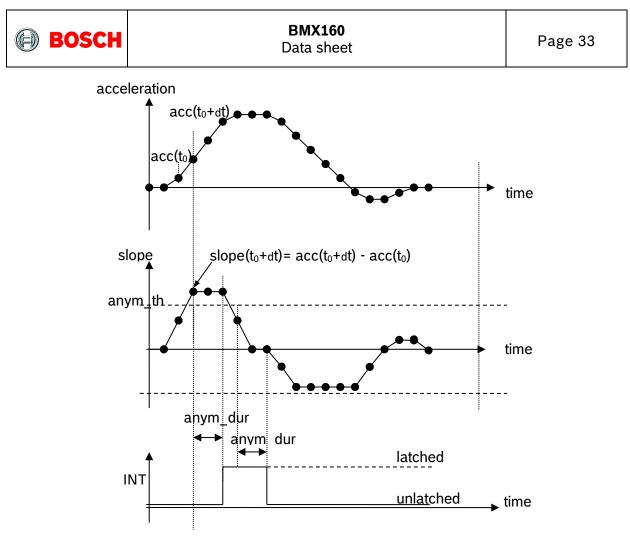
Figure 6: Any-motion (slope) interrupt detection
