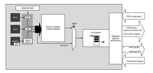
Figure 4: Block diagram of FIFO data path
