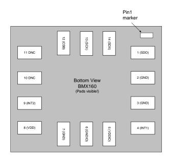
Figure 31: Pin-out bottom view
