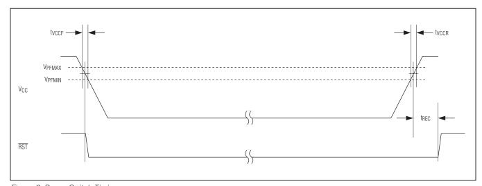
Figure 2. Power Switch Timing
