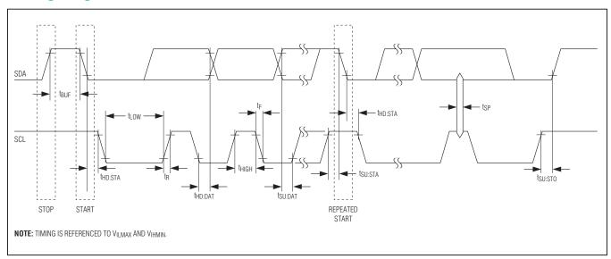
Figure 1. I<sup>2</sup>C Timing
