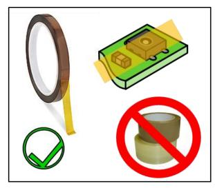
In conjunction with the sensor, use only recommended Kapton® tape Electrical Tape 92 by  $3M^{\text{TM}}$ .
