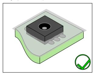
If conformal coating is applied, the top surface of the sensor must remain free of coating.
